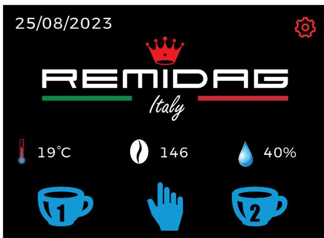
To adjust the supply time relating to the single dose, double and triple, you need to access SETTINGS menu, pressing red gear in the upper right corner of the screen.
